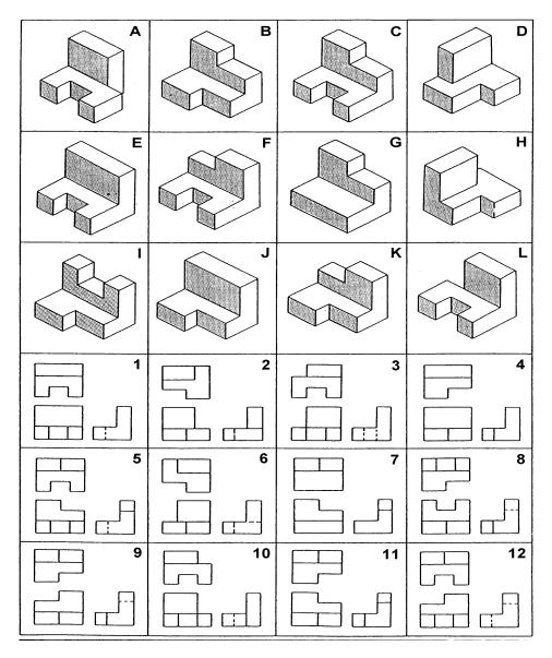
Pick the letter that of the isometric drawing that matches the orthographic projection.
